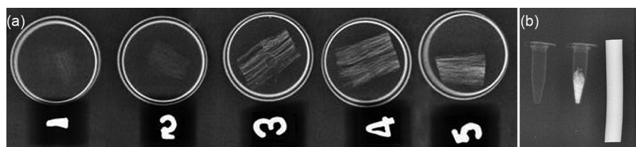
Figure 3. Radiograph showing X-ray opacity of the chitosan derivatives. (a) Fibrous sheets (average thickness of 1 mm) placed in the hollow aluminum rings of equivalent thickness (1, uncross-linked chitosan; 2, DHF cross-linked chitosan; 3, CDI 44 ; 4, CDI 85 ; 5 CDI 85 ) (3, 4, and 5 are chitosan fibrous sheets cross-linked with iodinated DHF, C = chitosan, D = DHF, and I = iodine, and the subscript = average opacity); (b) X-ray visibility of empty eppendorf, eppendorf containing radiopaque microsphere, CDI m , and commercially available radiopaque tape (from left to right).
